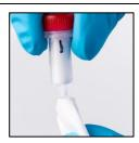
1.8 Add 50-200  $\mu$ L antibody solution (~100  $\mu$ g) slowly on the **top end** of the inclined resin bed.
