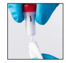
3.7 Add the protein labeling solution from Step 2.3 slowly on the **top end** of the resin and ensure that the resin is still inclined. In case of a sample volume  $< 70~\mu L$  add the antibody solution in the way described above and let the solution sink into the resin. Add an **additional amount of 15 \mu L** PBS buffer in the same way.
